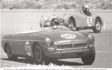
▲ Jim Adams in the HSC MGB. Note the changes HSC and Spencer made to the car for 1964 (Silverstone mag wheels, Spencer handmade cockpit tonneau and lower front valance brake ducts).
